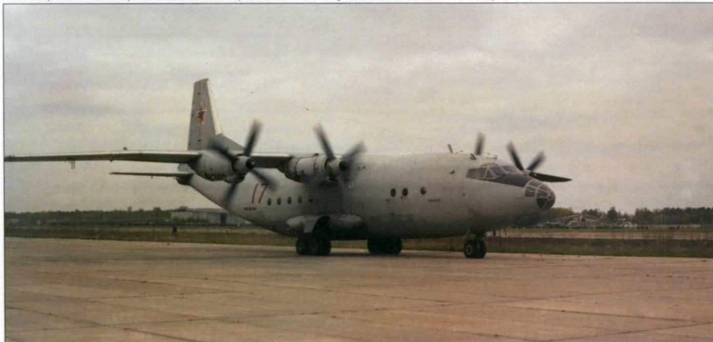
На земле большие створки носовой и основных опор закрыты / Being on the ground the aircraft has large NLG and MLG wheel well doors closed
